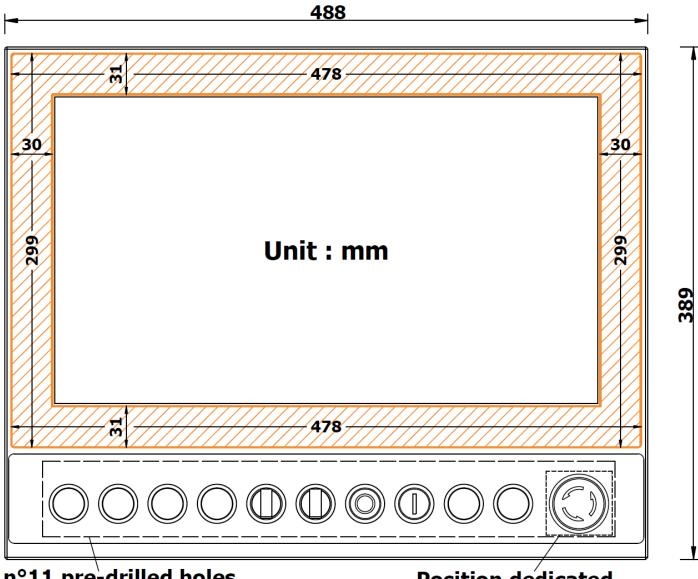
n°11 pre-drilled holes for Ø22 elements Position dedicated to a possible emergency button
