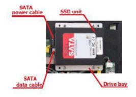
Unscrew the four screws marked above then unplug the two SATA cables. On the rear of the drive bay there are further four screws that lock the SSD unit.
