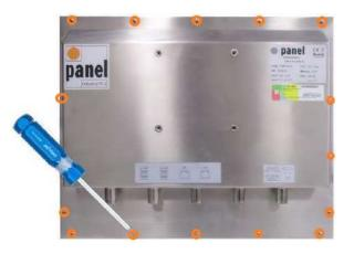
Unscrew all the screws used to hold the rear cover in place, and remove the rear cover.
