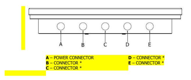
\*Connectors quantity and I/O connections depend by customer configurations
