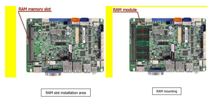
SO-DIMM slot supports one 204-pin DDR3 (Double Data Rate 3) single channel DDR3L SDRAM only.
