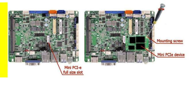
Mini PCI-E socket installation area
